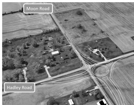
The roadway will be widened to include two full 12-foot lanes, with new turn lanes being installed at the school site. Improvements also include construction of an 8' pedestrian sidepath that will close an existing gap along the corridor, while also providing a new connection to the school. Street lighting and drainage improvements are also being incorporated into the project.
